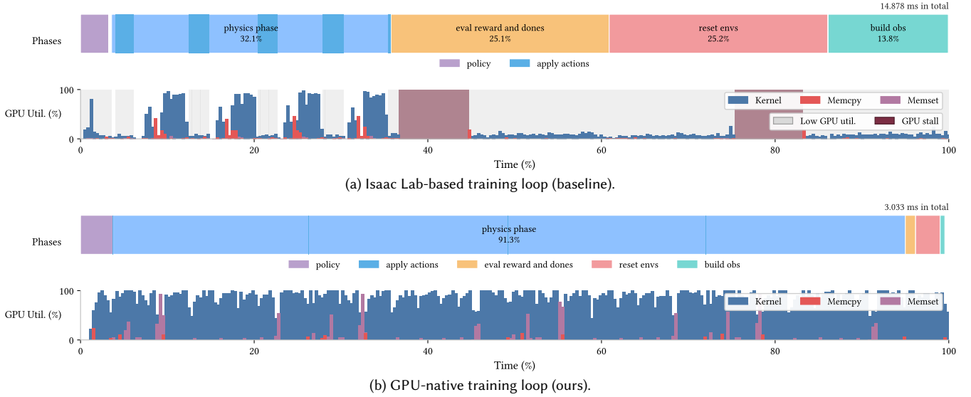
Fig. 2. GPU profiling timeline of a single rollout step in two PPO training loops.
